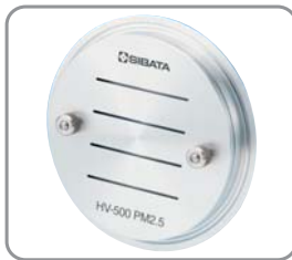
PM2.5 Impactor (2.5µm 50%Cut)
